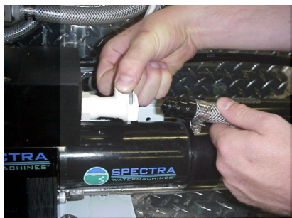
Connecting brine discharge service hose
