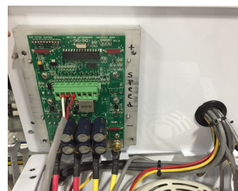
Motor speed controller DC (above the motor, under the lid of the box)
