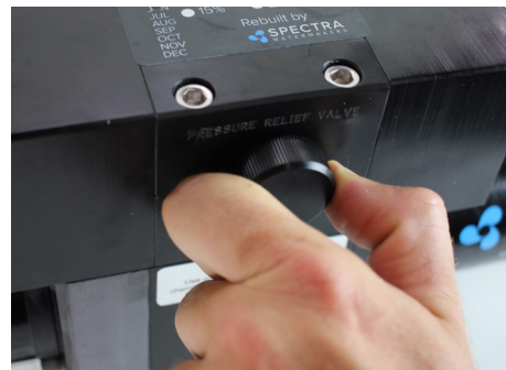
Open the Pressure Relief Valve
