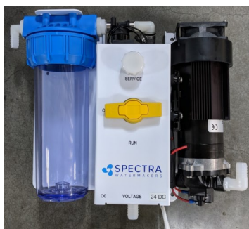
Service valve in OFF position
