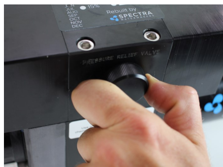
Open the pressure relief valve!
